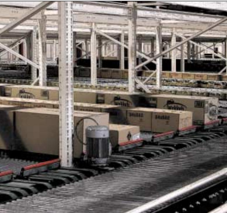
As products are carried along on the input lane, an input trolley at each level sees to it that the items are routed into the correct storage lane. The storage lanes are typically 40 feet long, which not only allows for a large area of entry for each product, but assures timely replenishment. The system is designed to handle items of all sizes, weights, and packaging types, including fragile products. (Fast-moving items are assigned to more than one storage lane.)
